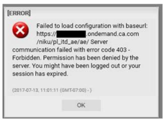
Cause: reference to the pl\_itd\_ae component removed from the components.xml file.
